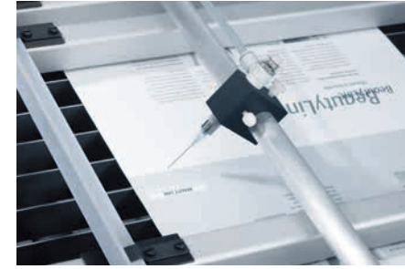
Wet scoring prevents thick folded products from 'popping up'.
